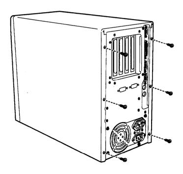
5. Grasp the sides of the cover and pull it straight back, until it clears the computer.
